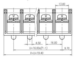
Recommended terminal lug should be suitable for M5 screw with outer width/diameter of <13 mm to fit inside housing. Additionally, the lug must support a maximum screw tightening torque of 2.4 N·m
