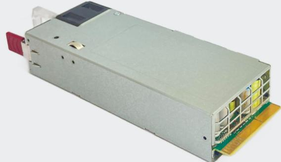
Advanced Energy's Artesyn CSU front end series is designed to provide a flexible power conversion solution for compute, storage, and networking equipment in the modular hardware common redundant power supply (M-CRPS). The 2400 W model is in the standard 1 U x 73.5 mm x 185 mm form factor. The series of power supply can cover cost-sensitive entry level systems, or power hungry applications where there are space constraints.
