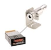
→ The supply voltage for DA 6000-N may be either 85 to 265 V AC or 18 to 30 V DC. So it can be used all over the world.
