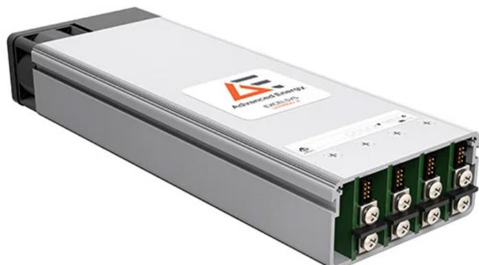
The approach leveraged proven success from previous applications for customers with similar systems. By customizing the XMC module which involved adjusting the Under Voltage Lockout (UVLO) detection settings and incorporating an AC voltage dip modification, the system achieved optimal performance while maintaining 2 MOPP safety compliance for medical standards.
