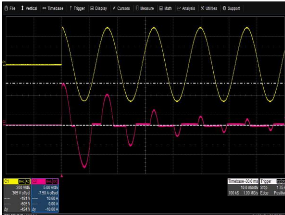
Figure 16: μMP09T-SKQ-S2Q-30-A Start up Inrush Current Vin = 264Vac Load: I O = 0A I SB = 0A Turn On Phase = 90° Ch 1: V IN Ch 2: I IN
