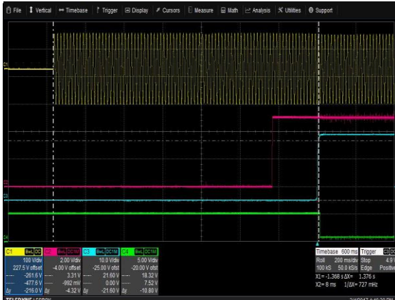
Figure 10: µMP09T-SKQ-S2Q-30-A Turn-on delay via AC mains Vin = 90Vac Load: I O = 23A I SB = 2A Ch 1: AC Mains Ch 2: V SB Ch 3: V O Ch 4: Global DCOK
