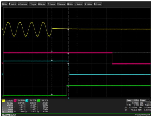
Figure 21: µMP10T-S2Q-S2Q-S2Q-S2Q-S2Q-90-A Hold-up Time via AC mains Vin = 90Vac/63Hz Load: I O = 41.66A I SB = 2A Ch 1: AC Mains Ch 2: V SB Ch 3: V O Ch 4: Global DCOK
