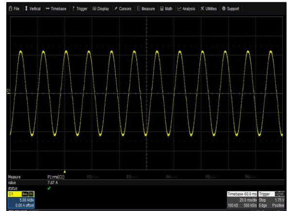
Figure 17: μMP09T-SKQ-S2Q-30-A Input Current Waveform Vin = 90Vac Load: I O = 23A I SB = 2A Ch 1: I IN
