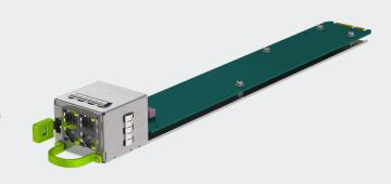
Advanced Energy's Artesyn<sup>™</sup> PMI is an extension module, which brings MODBUS of the PSU directly out for upstream communication. PMI sits on Open Rack V3 Power Shelves. On one end, it has communication with the PSU – through sliver straddle connector. On the other end, interacts with centralized system through the use of RJ45 connectors.
