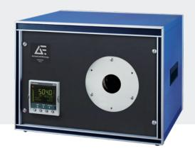
The Mikron® M305 blackbody calibration source uniquely combines portability with wide temperature range, high emissivity, and high accuracy. It is an ideal calibration unit where portability is required or where installation space is limited. Its spherical metal cavity design yields an emissivity of 0.995 over the temperature range of 100 to 1000°C (212 to 1832°F) with an aperture of 25 mm (1"). An integrally mounted PID controller adds to the unique versatility of this calibrator.
