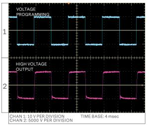
Figure D. 5HVA24-BP1 square wave input
