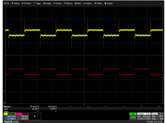
Figure 8: FCM10K Transient Response - Vo Deviation 75% to 100% load change, 1A/uS slew rate Vin = 480Vac Ch 1: Vo Ch 2: Io
