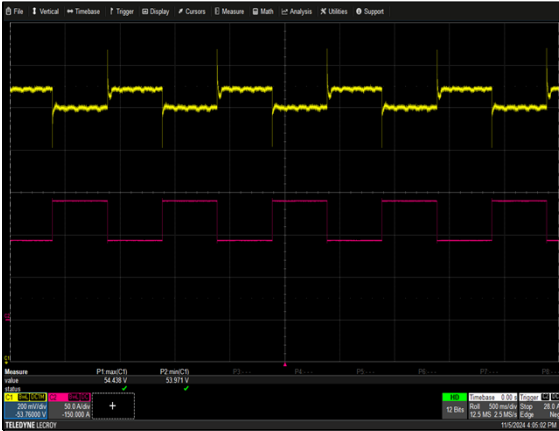
Figure 7: FCM10K Transient Response - Vo Deviation 50% to 75% load change, 1A/uS slew rate Vin = 480Vac Ch 1: Vo Ch 2: Io
