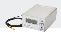
The Trek® 541A electrostatic voltmeter provides accurate non-contacting measurements of the electrostatic surface voltage associated with EOS/ESD processes. The instrument is configured with a miniature electrostatic field chopper probe that can be remotely located and easily positioned within process equipment to provide highly accurate, non-contacting, DC-stable, spacing-independent voltage measurements in either ionized or non-ionized environments.
