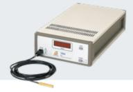
The Trek® 370 precision electrostatic voltmeter for non-contacting surface voltage measurements in the range of 0 to ±3 kV DC or peak AC. The Trek 370 employs an electrostatic field-nulling technique which achieves high DC stability and high measurement accuracy even if the probe to measured surface spacing changes. This permits measurements of either stationary or moving surfaces without the need to establish fixed spacing to maintain accuracy.
