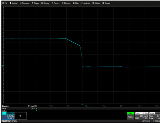
Figure 19: NCF250S24K Turn Off Characteristic V_{in} = 90VAC Load: I_o = 10.4A I_{SB} = 1A Ch 3: V_O
