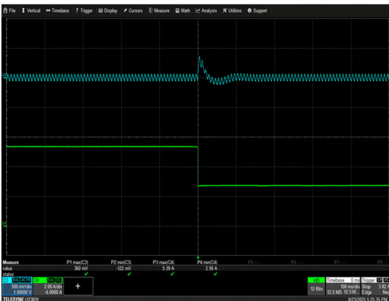
Figure 33: NCF250S48K Transient Response - V_o Deviation 100% to 50% load change 0.2A/\mu s slew rate, V_{in} = 230VAC Ch 1: V_o Ch 2: I_o
