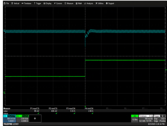
Figure 32: NCF250S48K Transient Response - V_o Deviation 50% to 100% load change 0.2A/\mu s slew rate, V_{in} = 230VAC Ch 3: V_o Ch 4: I_o
