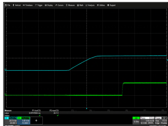
Figure 18: NCF250S24K Output Voltage Startup Characteristic V_{in} = 90VAC Load: I_o = 10.4A I_{SB} = 1A Ch 3: V_O Ch 4: DC_OK
