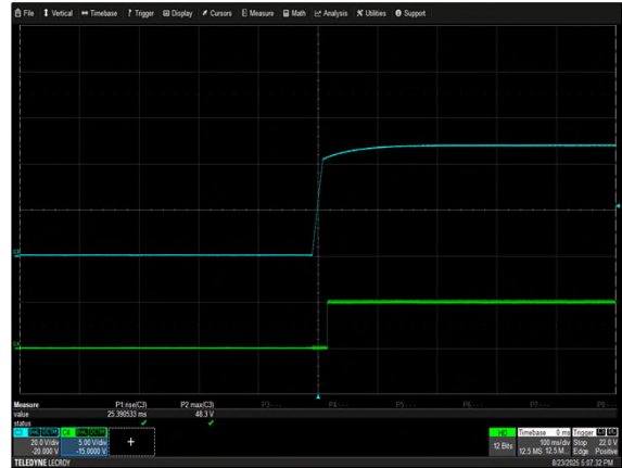
Figure 30: NCF250S48K Output Voltage Startup Characteristic V_{in} = 90VAC Load: I_O = 5.2A I_{SB} = 1A Ch 3: V_O Ch 4: DC_OK
