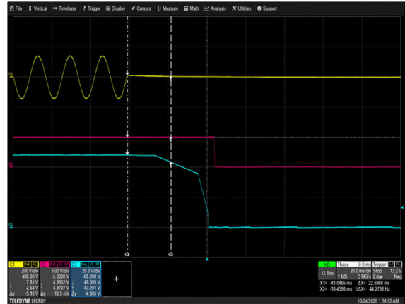
Figure 26: NCF250S48K Hold-Up Time V_{in} = 100VAC Load: I_O = 4.42A (85% load) I_{SB} = 1A Ch 1: V_{IN} Ch 2: V_{SB} Ch 3: V_O
