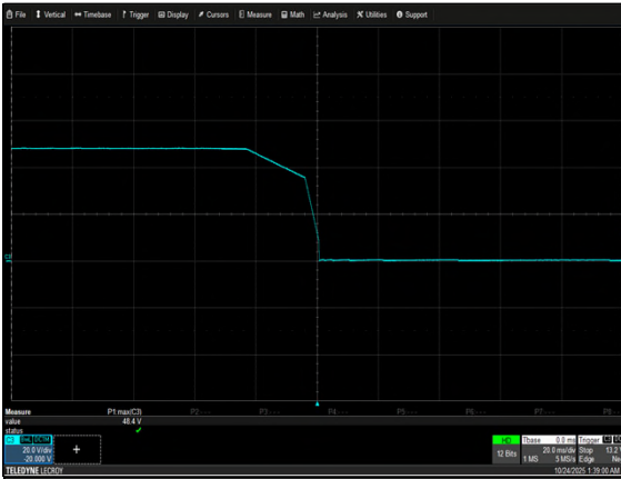
Figure 31: NCF250S48K Turn Off Characteristic V_{in} = 90VAC Load: I_o = 5.2A I_{SB} = 1A Ch 3: V_o
