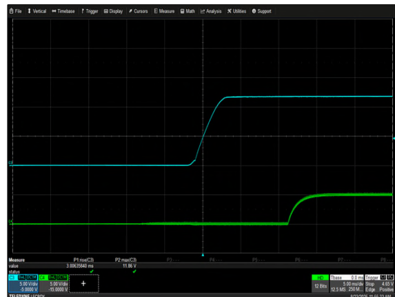
Figure 6: NCF250S12K Output Voltage Startup Characteristic V_{in} = 90VAC Load: I_O = 19.1A I_{SB} = 1A Ch 3: V_O Ch 4: DC_OK
