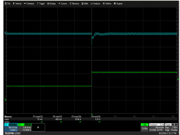
Figure 20: NCF250S24K Transient Response - V_O Deviation 50% to 100% load change 0.2A/\mu S slew rate, V_{in} = 230VAC Ch 3: V_O Ch 4: I_o
