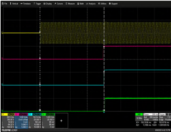
Figure 1: NCF250S12K Turn-On Delay via AC Mains V_{in} = 115VAC Load: I_O = 19.1A I_{SB} = 1A Ch 1: V_{IN} Ch 2: V_{SB} Ch 3: V_O Ch 4: DC_OK
