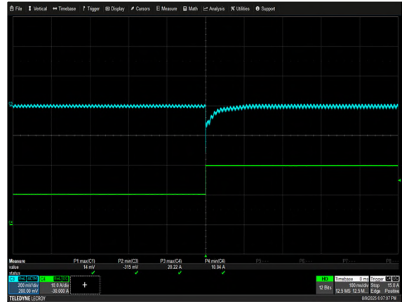
Figure 8: NCF250S12K Transient Response - V_o Deviation 50% to 100% load change 0.2A/\mu s slew rate, V_{in} = 230VAC Ch 3: V_o Ch 4: I_o
