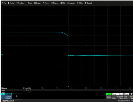
Figure 7: NCF250S12K Turn Off Characteristic V_{in} = 90VAC Load: I_o = 19.1A I_{SB} = 1A Ch 3: V_o
