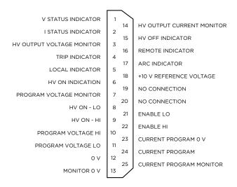
All logical indicators are open collector outputs rated at 16 V (max) in the OFF state. An internal 100  $\Omega$  resistor is connected in series with the open collector transistor. The pull down voltage is 0.9 V plus the internal resistor drop. The rated current is 10 mA.
