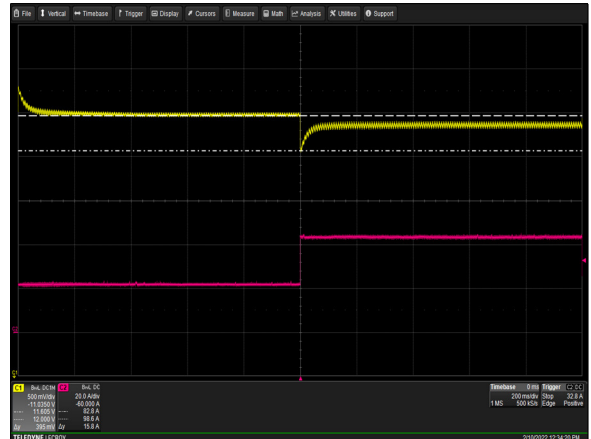
Figure 10: AIF42BAC-01N Transient Response - V O Deviation 50% to 100% load change 1A/μs slew rate Vin = 230Vac Ch 1: V O Ch 2: I O
