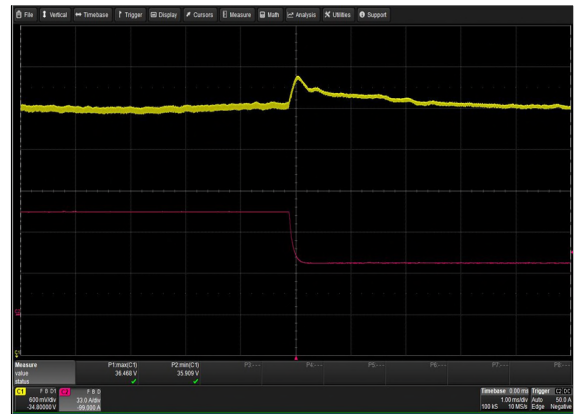
Figure 52: LCM3000U-T Transient Response - V_o Deviation 100% to 50% load change 1A/ \mu s slew rate V_{in} = 230V_{ac} Ch 1: V_o Ch 2: I_o
