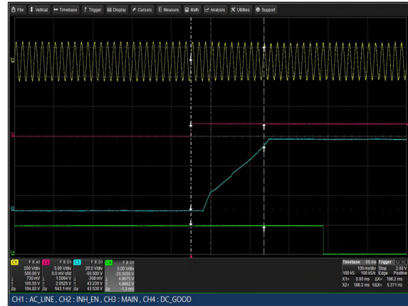
Figure 58: LCM3000W-T Turn-on delay via INH_EN Vin = 90Vac Load: Io = 31.25A (48V), Isb = 2A Ch 1: Vin Ch 2: INH_EN Ch 3: Vo Ch 4: G_DCOK_C
