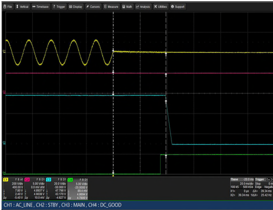
Figure 61: LCM3000W-T Hold-up Time Vin = 90Vac Load: Io = 31.25A (48V), Isb = 2A Ch 1: Vin Ch 2: Vsb Ch 3: Vo Ch 4: G_DCOK_C
