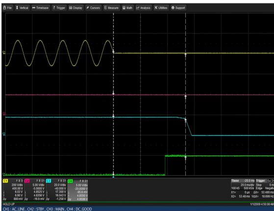
Figure 19: LCM30008-T Hold-up Time Vin = 90Vac Load: Io = 83.3A (18V), Isb = 2A Ch 1: Vin Ch 2: Vsb Ch 3: Vo Ch 4: G_DCOK_C
