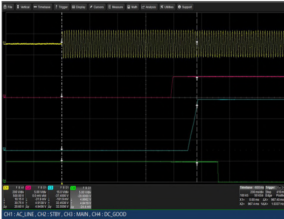
Figure 43: LCM3000U-T Turn-on delay via AC mains Vin = 90Vac Load: Io = 41.7A (36V), Isb = 2A Ch 1: Vin Ch 2: Vsb Ch 3: Vo Ch 4: G_DCOK_C
