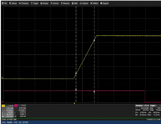
Figure 21: LCM30008-T Output Voltage Startup V_{in} = 264V_{ac} Load: I_o = 166.7A (18V), I_{sb} = 2A Ch 1: V_o Ch 2: G\_DCOK\_C
