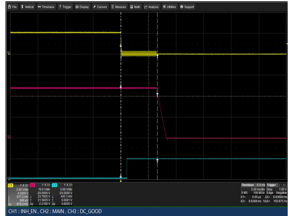
Figure 36: LCM3000Q-T Turn Off Characteristic via INH_EN Vin = 264Vac Load: Io = 125A (24V), Isb = 2A Ch 1: INH_EN Ch 2: Vo Ch 3: G_DCOK_C
