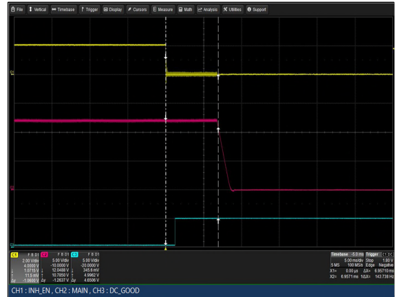
CH1: INH_EN, CH2: MAIN, CH3: DC_GOOD Figure 8: LCM3000L-T Turn Off Characteristic via INH_EN Vin = 264Vac Load: Io = 125A (12V), Isb = 2A Ch 1: INH_EN Ch 2: Vo Ch 3: G_DCOK_C
