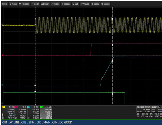
Figure 57: LCM3000W-T Turn-on delay via AC mains Vin = 90Vac Load: Io = 31.25A (48V), Isb = 2A Ch 1: Vin Ch 2: Vsb Ch 3: Vo Ch 4: G_DCOK_C
