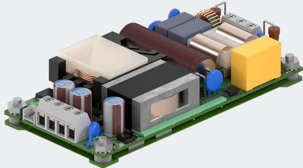
Advanced Energy's SL Power LPP200 AC-DC are low profile (0.75") open frame power supplies suitable for many medical and industrial applications where space is at a premium.
