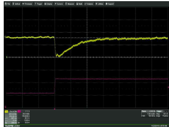
Figure 8: CSU550AP-3 Transient Response - V_O Deviation (low to high)
