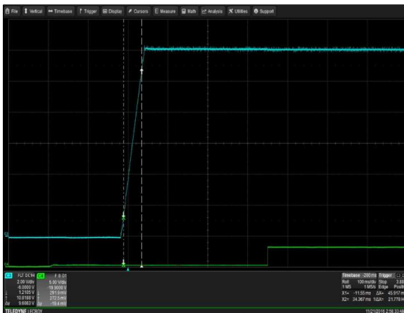
Figure 5: CSU550AP-3 Output Voltage Startup Characteristic
