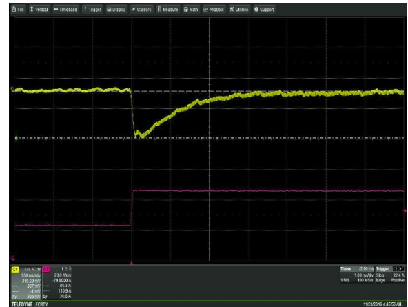
Figure 8: CSU550AP-3 Transient Response - V_o Deviation (low to high) 50% to 100% load change, 0.25A/\mu S slew rate, V_{in} = 230Vac Ch 1: V_o Ch 2: I_o
