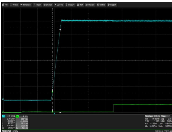
Figure 5: CSU550AP-3 Output Voltage Startup Characteristic Vin = 90VAC Load: Io = 45A I SB = 2.5A Ch 3: V O Ch 4: PWOK
