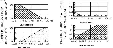
EFFECTS OF LOAD RESISTANCE AND CAPACITANCE AT 400 Hz
