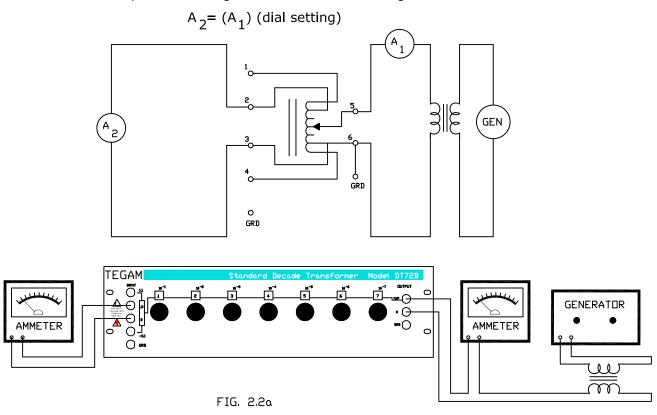
In current divider applications a negligible voltage should appear across the input impedance of the DEKATRAN. The graph in Figure 2.2b gives the error due to the impedance of the ammeter for ammeter resistances from 10 milliohms to 100 ohms.
