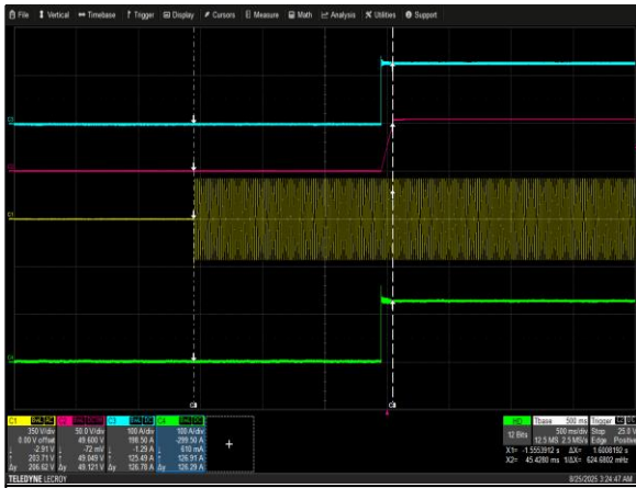
Figure 1: FCM30K Turn-on delay via AC mains Vin = 208VAC Load: Io = 251A Ch 1: Vin Ch 2: Vo Ch 3: Io 1 Ch 4: Io 2
