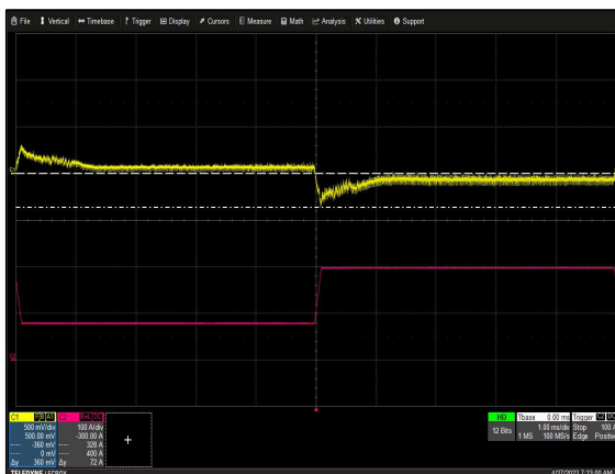
Figure 11: CSU2400AT-3-100 Transient Response - V_O Deviation 40% to 100% load change 0.5A/μs slew rate V_{in} = 230V_{ac} Ch 1: V_O Ch 2: I_O
