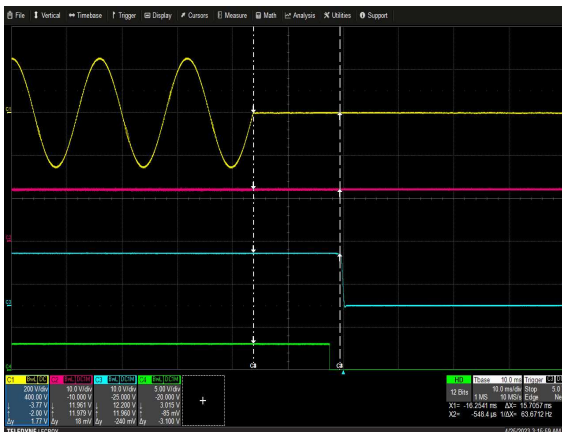
Figure 3: CSU2400AT-3-100 Hold-Up Time V_{in} = 180V_{ac} Load: I_O = 196.7A I_{SB} = 3.5A Ch 1: AC Mains Ch 2: V_{SB} Ch 3: V_O Ch 4: PWOK
