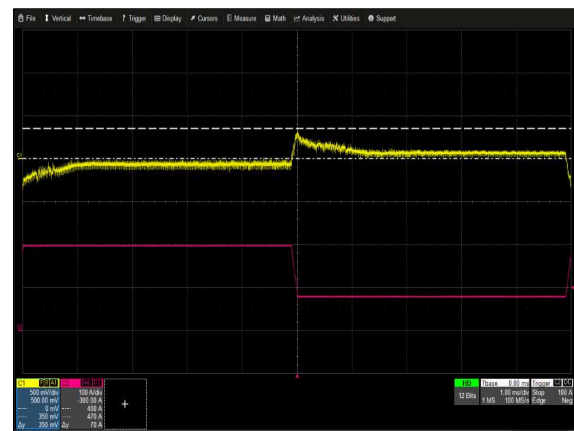
Figure 12: CSU2400AT-3-100 Transient Response - V_O Deviation 100% to 40% load change 0.5A/μs slew rate V_{in} = 230V_{ac} Ch 1: V_O Ch 2: I_O
