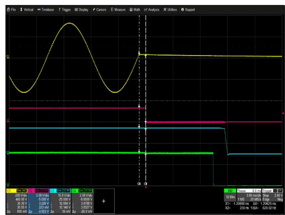
Figure 6: CSU2400T-3-100 VIN_GOOD De-assert Characteristic V_{in} = 230V_{ac} Load: I_O = 196.7A I_{SB} = 3.5A Ch 1: AC Mains Ch 2: VIN_GOOD Ch 3: V_O Ch 4: PWOK
