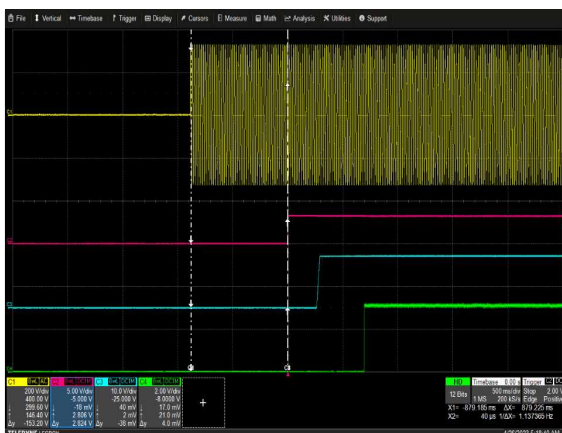
Figure 5: CSU2400AT-3-100 VIN_GOOD Assert Characteristic V_{in} = 230V_{ac} Load: I_O = 196.7A I_{SB} = 3.5A Ch 1: AC Mains Ch 2: VIN_GOOD Ch 3: V_O Ch 4: PWOK
