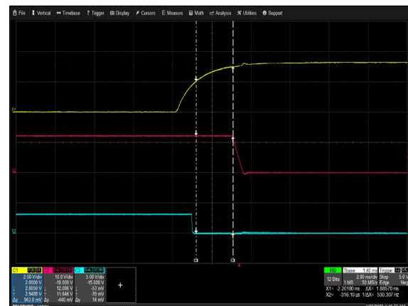
Figure 10: CSU2400AT-3-100 Turn Off Characteristic via PSON V_{in} = 264V_{ac} Load: I_o = 196.7A I_{SB} = 3.5A Ch 1: PSON Ch 2: V_O Ch 3: PWOK
