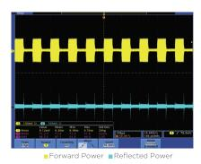
Navigator® II matching network: Advanced algorithms allow for active tuning during a pulse.
