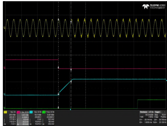
Figure 2: DS1100SLPE-3 Turn-On Delay via PSON
