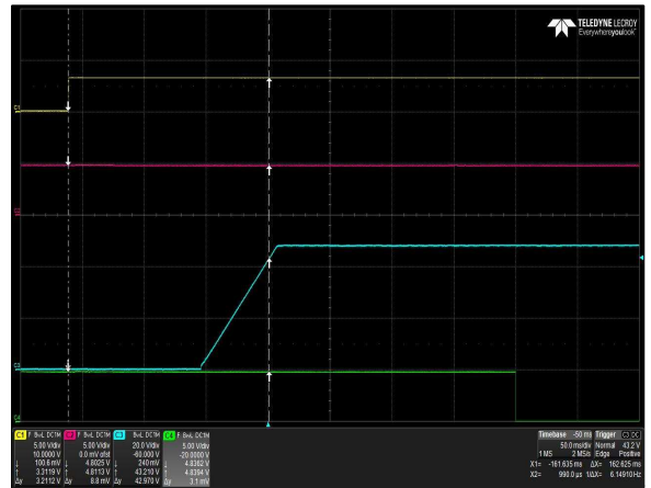
Figure 72: LCC600-48H-9P Turn-on delay via INH_EN Vin = 180Vac Load: I O = 12.5A (48V), I SB = 1.5A (5V) Ch 1: INH_EN Ch 2: V SB Ch 3: V O CH 4: G_DCOK_C
