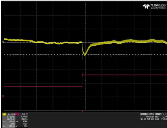
Figure 47: LCC600-36U-9P Transient Response - V_O Deviation 50% to 100% load change 1A/uS slew rate V_{in} = 230V_{ac} Ch 1: V_O Ch 2: I_O
