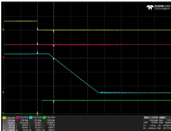
Figure 29: LCC600-28U-9P Turn Off Characteristic via INH_EN Load: I_O = 21.5A (28V), I_{SB} = 1.5A (5A) Ch 1: INH_EN Ch 2: V_{SB} Ch 3: V_O CH 4: G_DCOK_C
