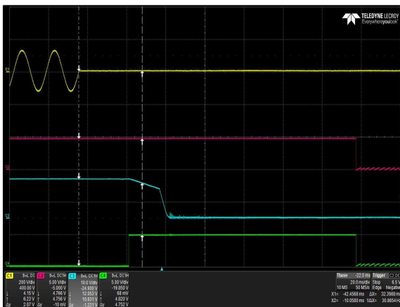
Figure 3: LCC600-12U-9P Hold-up Time Vin = 90Vac / 63Hz / 0° Load: Io = 50A (12V), I SB = 1.5A (5V) Ch 1: AC Mains Ch 2: V SB Ch 3: V O CH 4: G_DCOCK_C
