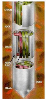
Figure 5 – The GTSM Tensor Strainmeter as installed in the borehole.
