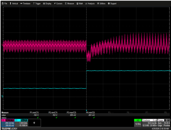
Figure 28: NCF660S48K Transient Response - Vo Deviation Vin = 115VAC Load: Io = 25% to 75%, 0.2A/ \mu s slew rate Ch 2: Vo Ch 3: Io
