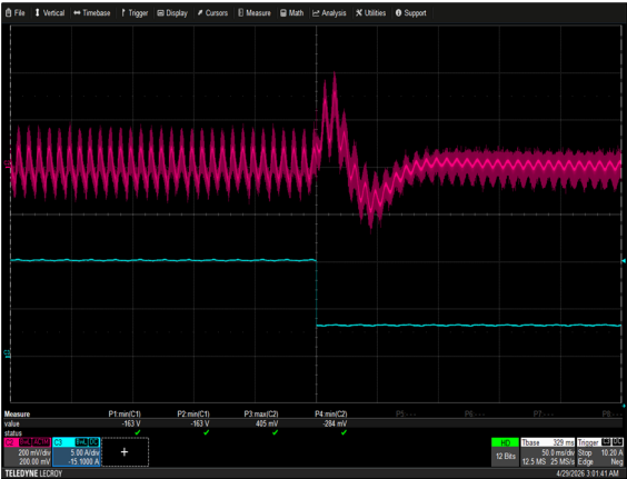
Figure 27: NCF660S48K Transient Response - Vo Deviation Vin = 115VAC Load: Io = 75% to 25%, 0.2A/ \mu s slew rate Ch 2: Vo Ch 3: Io
