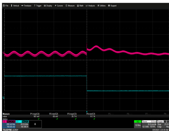
Figure 7: NCF660S12K Transient Response - V_o Deviation V_{in} = 115VAC Load: I_o = 75\% to 25\% , 0.2A/\mu s slew rate Ch 2: V_o Ch 3: I_o
