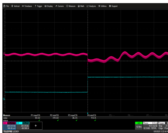
Figure 8: NCF660S12K Transient Response - V_o Deviation V_{in} = 115VAC Load: I_o = 25\% to 75\% , 0.2A/\mu s slew rate Ch 2: V_o Ch 3: I_o
