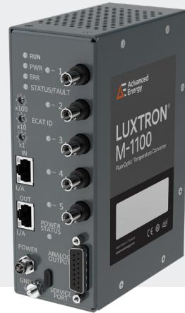
The Advanced Energy's Luxtron® M-1100 is the latest FluorOptic® thermometry (FOT) converter platform, featuring an advanced light source and improved ultralow noise electronics. Two new proprietary phosphor formulations VioLux™ and RubiLux™ have been developed to deliver 0.5°C accuracy, repeatability, and stability over an extended range -200 to 450°C.
