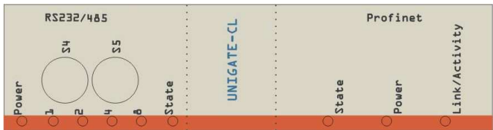
Picture 2: Front panel: Rotary switches and LEDs
