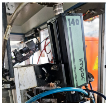
AE pyrometers mounted in equipment used as part of Tenneco's hardening and tempering processes.
