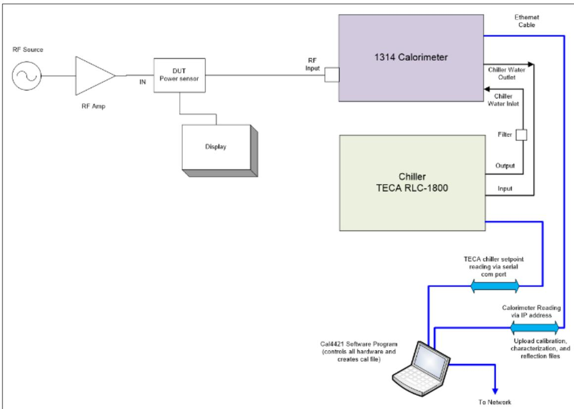
Figure 18: Manual RF Calibration Set-up
