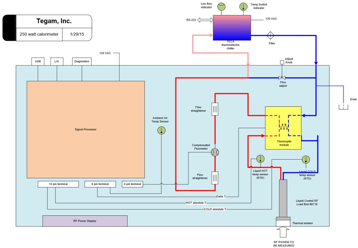
Figure 4: Signal Processing Block Diagram
