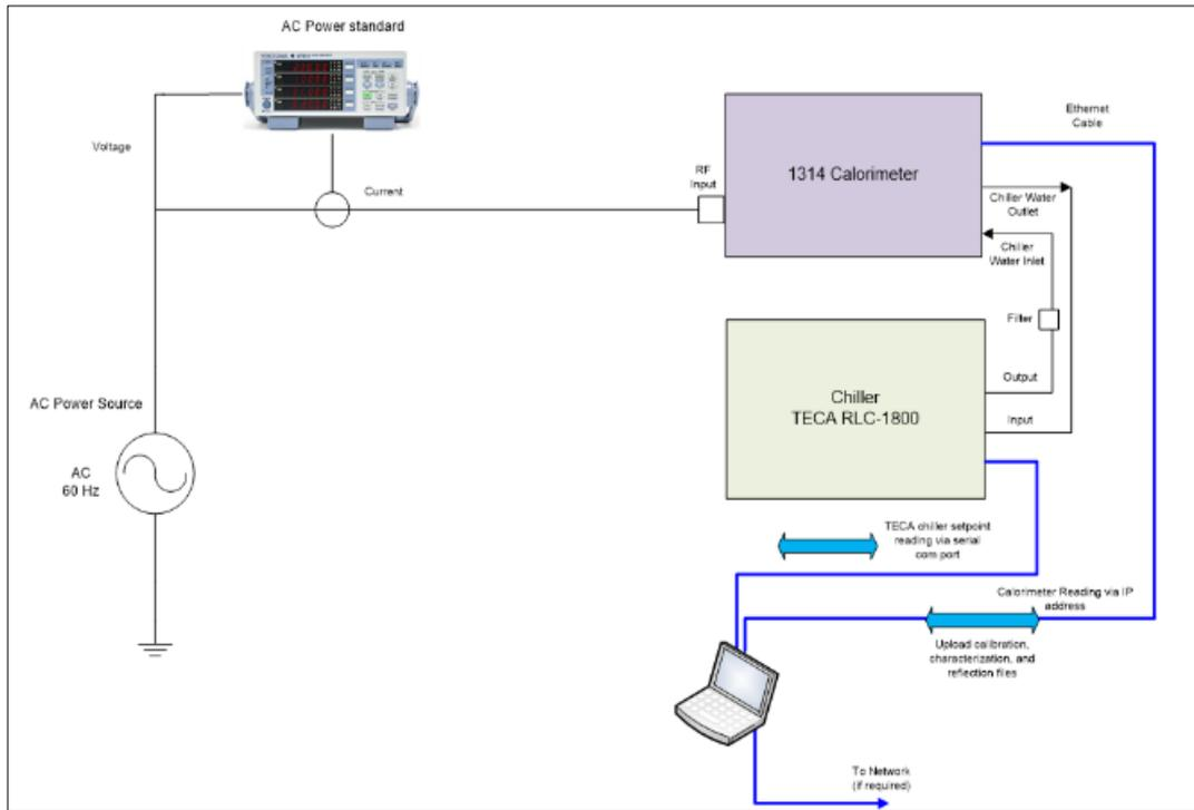
Figure 17: Manual AC Calibration Configuration
