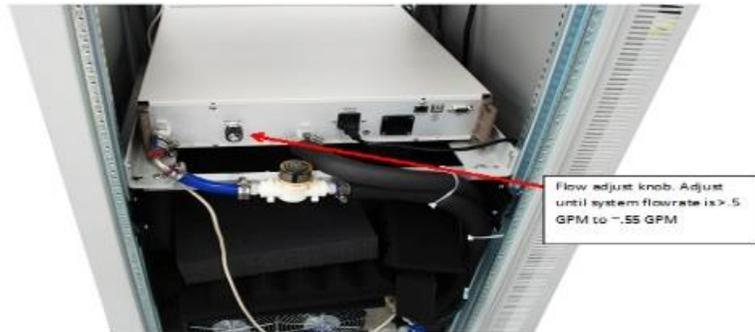
Figure 12: Flow adjustment knob
