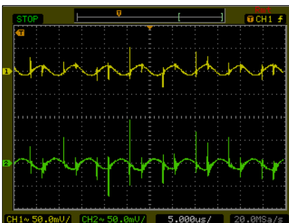
Figure 91: ASA01CC48-M Ripple and Noise Measurement Vin = 48Vdc Load: Io = ± 0.2A Ch 1: Vout1 Ch 2: Vout2
