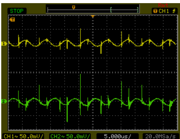
Figure 83: ASA01BB48-M Ripple and Noise Measurement Vin = 48Vdc Load: Io = ± 0.25A Ch 1: Vout1 Ch 2: Vout2
