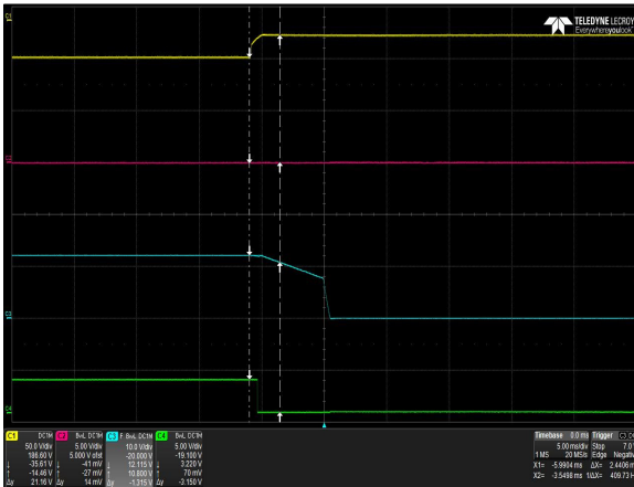
Figure 3: DS1100SDC-3 Hold-up Time Vin = -36Vdc Load: I_O = 91.6A I_{SB} = 3A Ch 1: Vin Ch 2: V_{SB} Ch 3: V_O Ch 4: Pwr_Good
